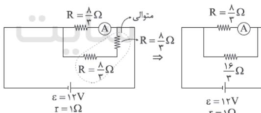
$$R'_{eq} = \frac{\frac{1}{3} \times \frac{16}{3}}{\frac{1}{3} + \frac{16}{3}} = \frac{\frac{16}{9}}{\frac{24}{3}} = \frac{16}{8 \times 3} = \frac{16}{9} \Omega$$
