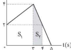
$$\left\{ \begin{array}{l} S_1 = \frac{4+2}{2} \times 3 = 9\text{m} \\ S_2 = \frac{4+2}{2} \times 1 = 3\text{m} \end{array} \right.$$
